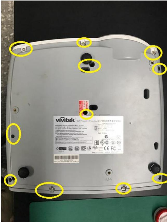
Remove the 4 back screws holding the connectors:
