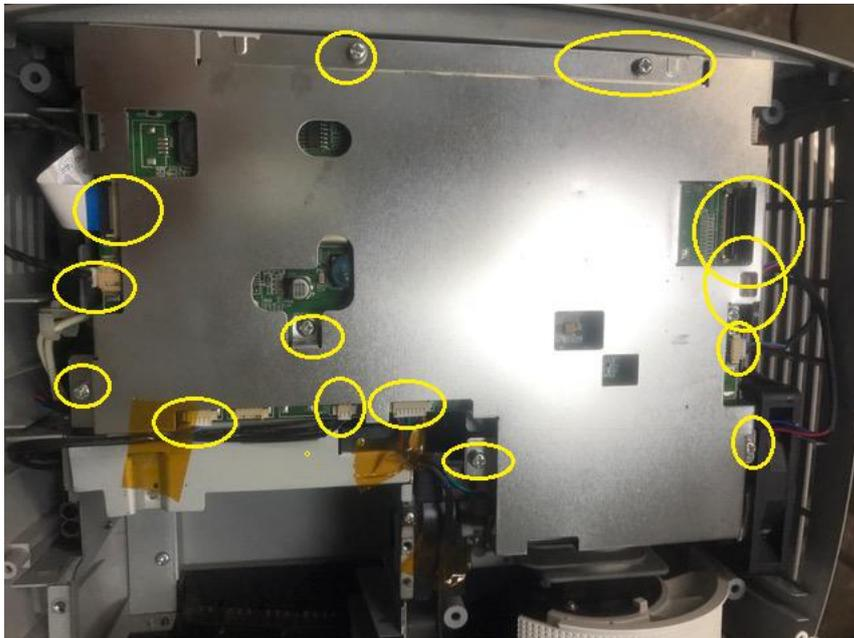
Remove the PCB screws:
