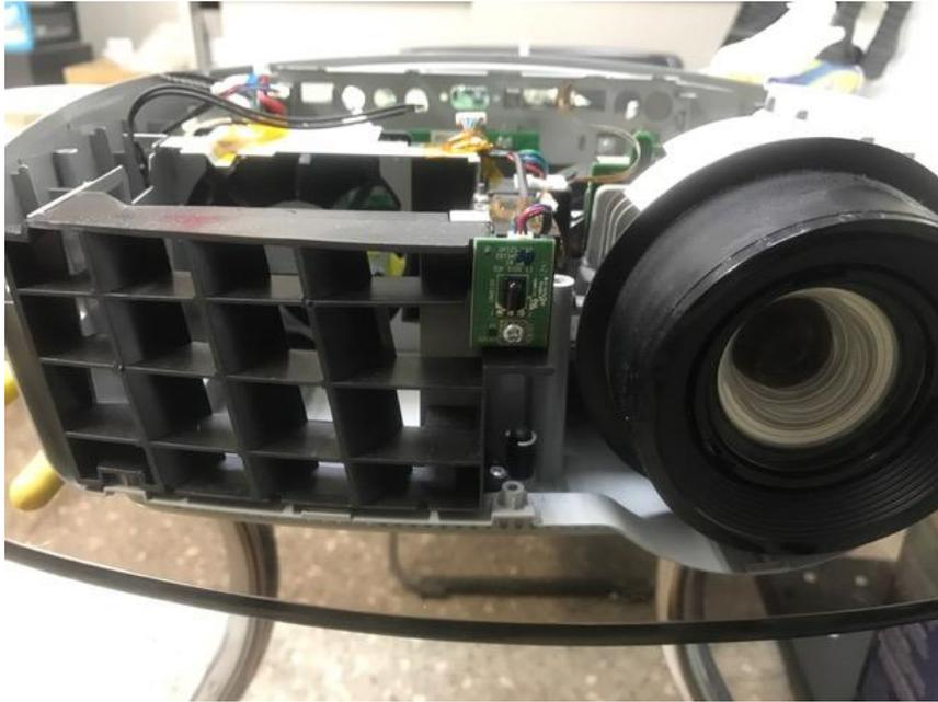
Remove the optical engine screws:
