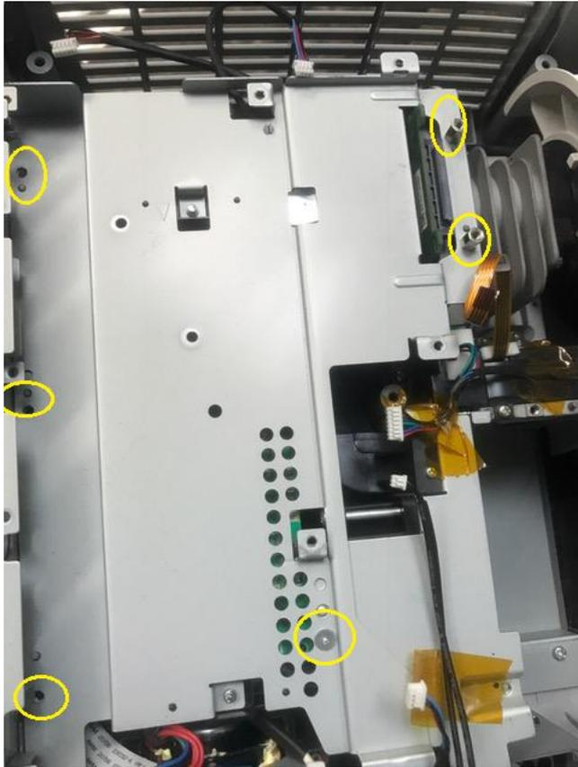
Pull the back of the projector out a few mm gently so the metal cover can clear the back and lift up on the metal cover:
