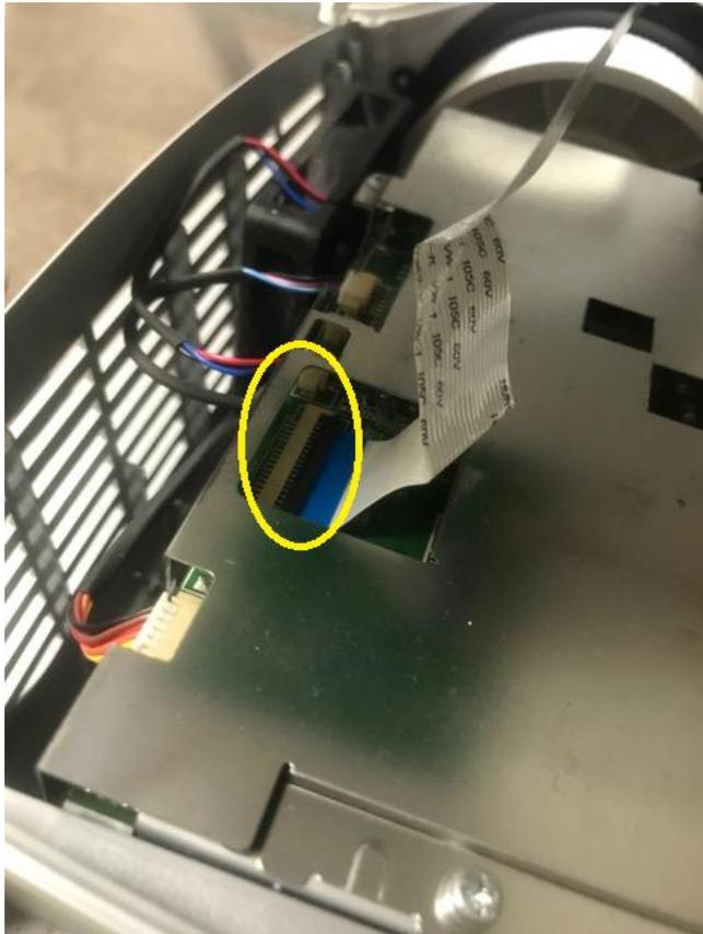
Unplug the connectors. Remove the screws from the metal cover:
