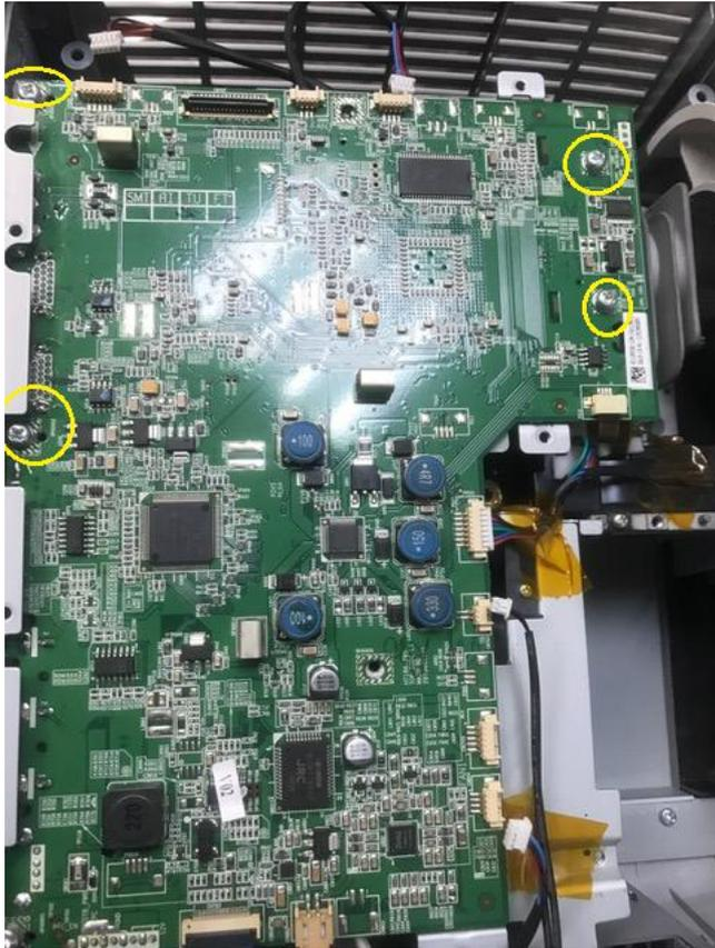
Lift it up a couple cm and remove the connector(s):
